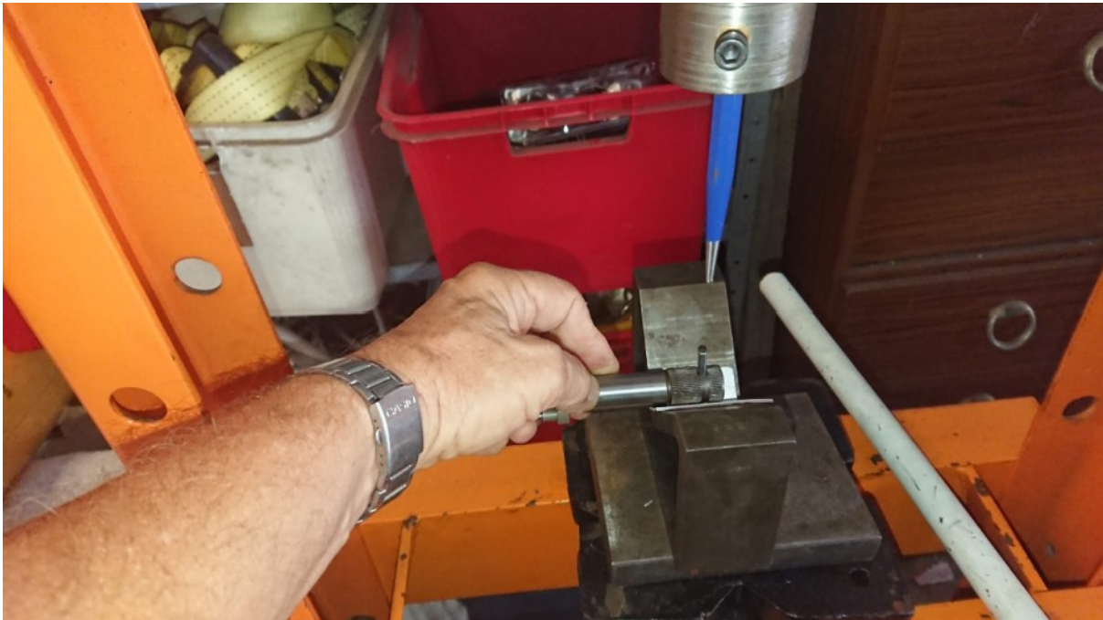
Press with punch in, shaft resting on aluminium packers in V block
