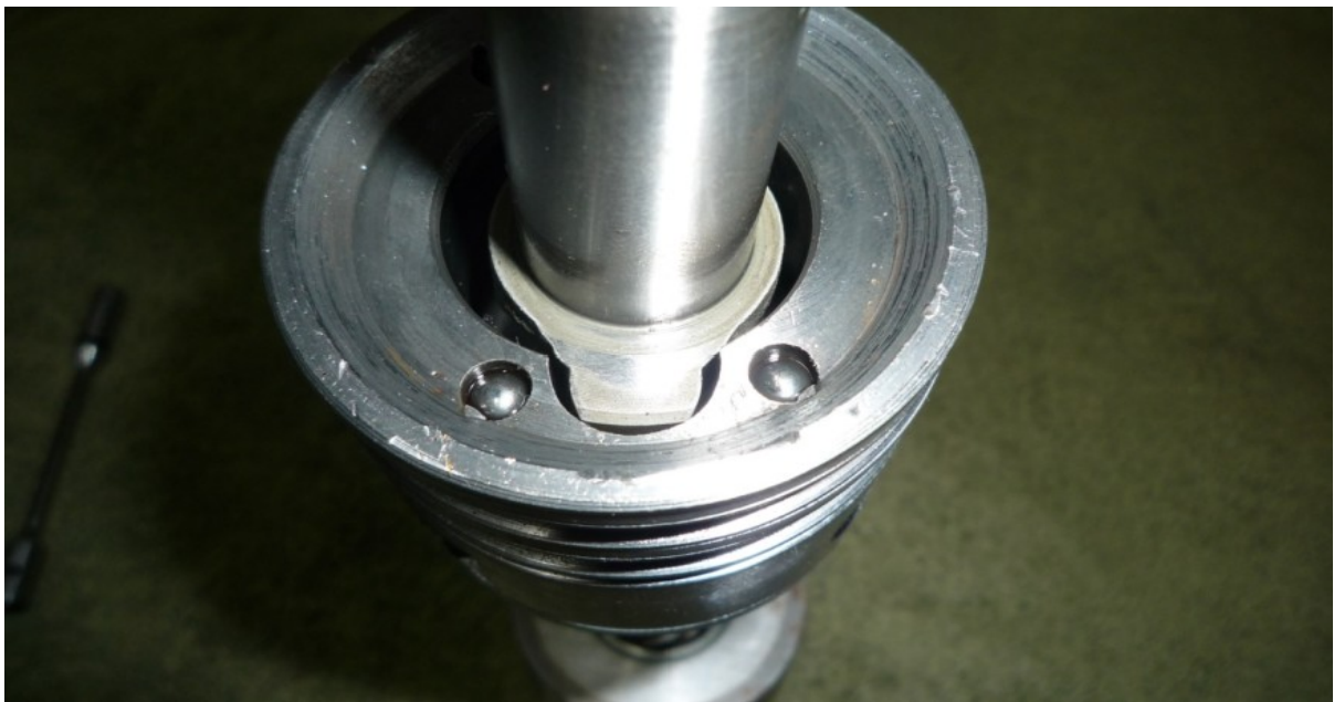
Small angular movement between input shaft (top) and pinion shaft (bottom)
