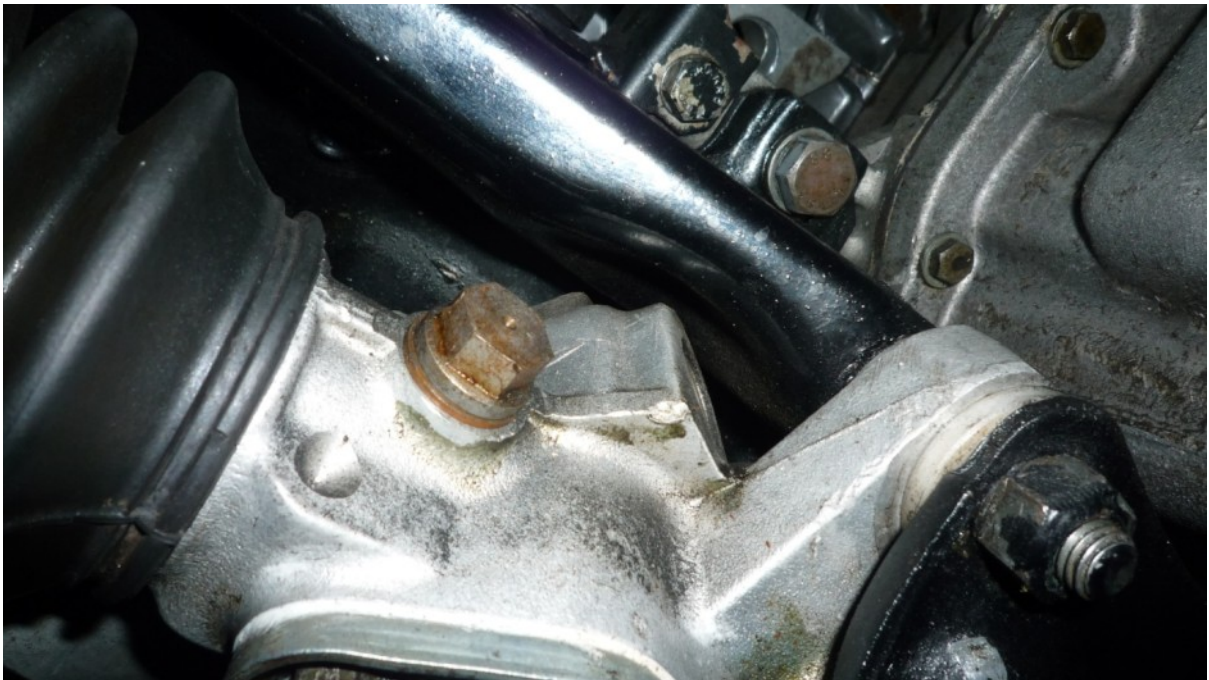
Rack centring inspection hole
