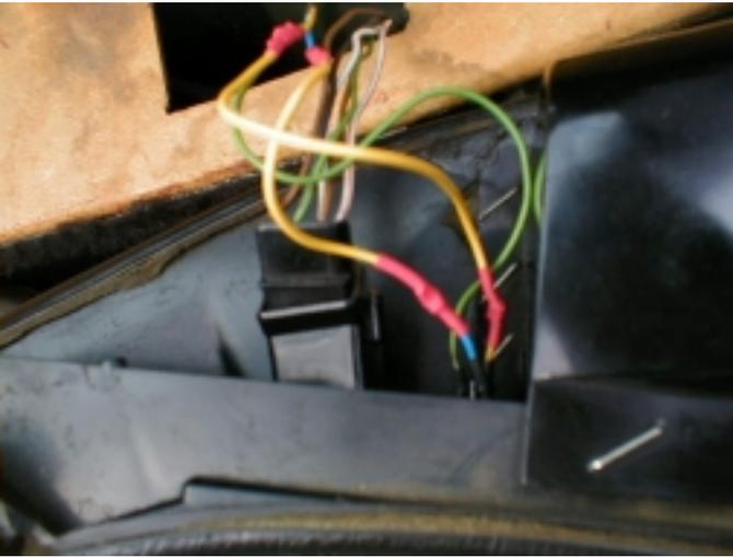
but on the driver's side panel when you remove the armrest you should just tilt it towards you some, exposing the [wires](#) on the underside of the power mirror switch (and seat position memory switch if you have it - I don't). Just unplug the wires. Make sure you keep track of which wires connect where on the crossover switch in front of the power mirror switch.
