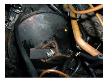
Then clamp the push rod at the master cylinder end to stop it retracting. I loosened the end piece on the pushrod pedal. I then inserted the pin from the other side and lodged the square end face of push rod block against the pin so I could use the brake pedal to push the booster plunger to the end of its travel in the booster and then clamp it there on the engine bay side. See pic below.
