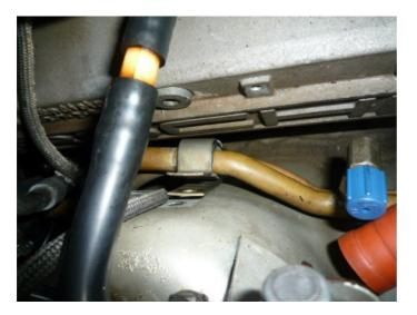
Undo the securing clip on the air-con rigid pipes securing them to the suspension turret to allow a little springiness.
