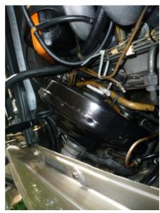
Continue to rotate the booster anticlockwise as in the photos until you can wriggle it out. The photo immediately above shows the angle of the booster for final removal or initial insertion if putting it back in.
