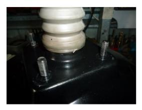
When the booster is bolted in release the pushrod clamp, fit the locknut and push rod end piece, adjust the length of the rod as per Workshop Manual (just a little play with push rod fully back against the internal stop in the booster). Grease and insert the pivot pin and don't forget the pedal return spring.
